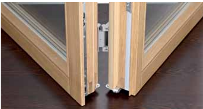
Height-adjustable sash hinges, view from inside; the caps of the sash hinges can only be removed in the open position
